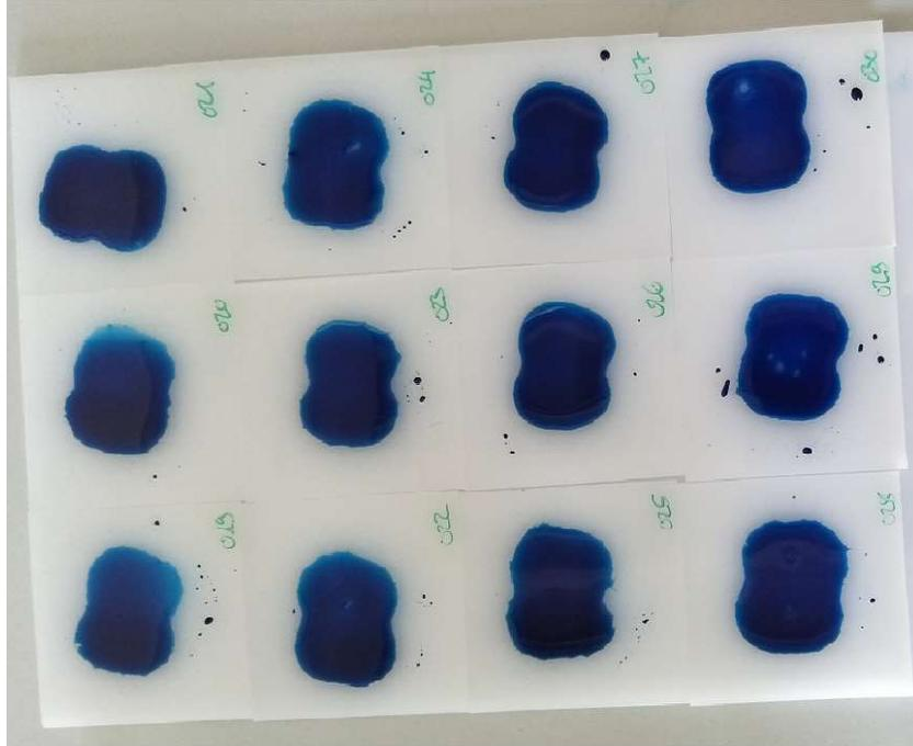
Figure 5: The activation areas visualized by 58 mJ/m<sup>2</sup> test ink on three HDPE substrates per module treated by piezobrush<sup>®</sup> PZ3 with standard modules 5942-0697 to 5942-0892, as listed in the table in Figure 1 after 6000 h of endurance test.
