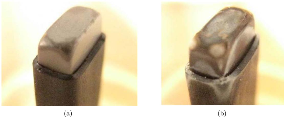
Figure 11: The tip of the CeraPlas<sup>®</sup>F from the standard module a) before and b) after 6000 operation hours.
