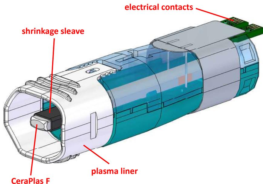
Figure 1: The mockup of the piezobrush<sup>®</sup> PZ3 standard module.
