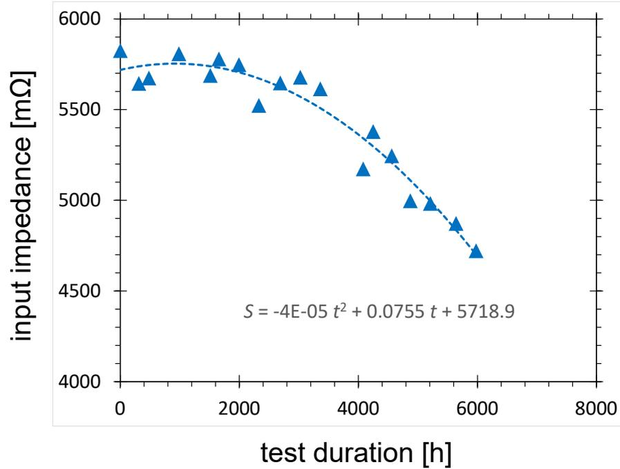
Figure 8: The CeraPlas<sup>®</sup> F input impedance as a function of endurance test duration. Each point in the diagram represents the average value for 10 modules.
