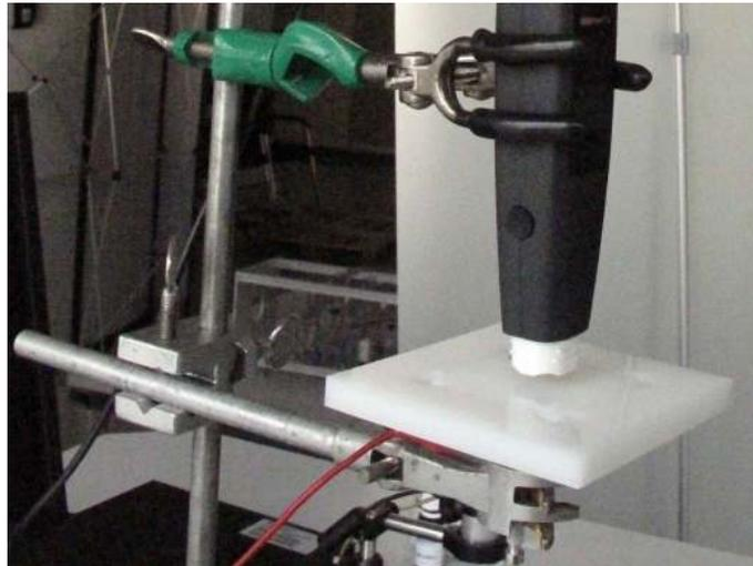
Figure 3: The HDPE substrate positioned on the HDPE substrate holder under the standard module of the piezobrush<sup>®</sup> PZ3 prepared for plasma treatment.
