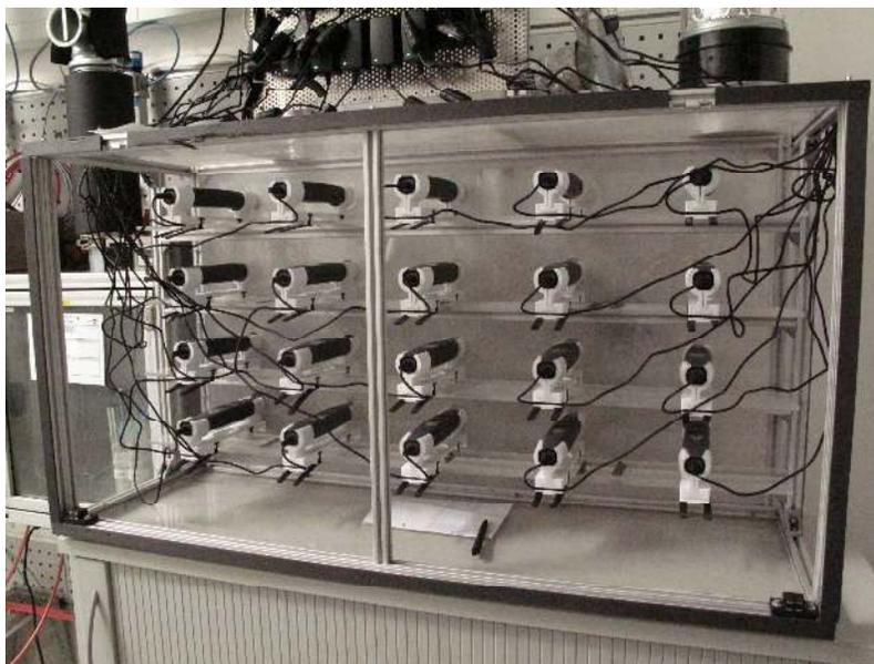
Figure 2: The cabinet for endurance test is equipped with 20 piezobrush<sup>®</sup>PZ3 fixed in digitally printed holders designed for operation with ten standard and ten near-field modules.
