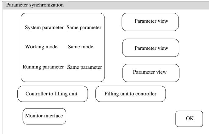
In main interface, click parameter synchronization button, to enter the synchronization interface.
