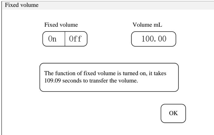
Click Fixed volume button to enter to set parameter interface for the fixed volume in main interface.
