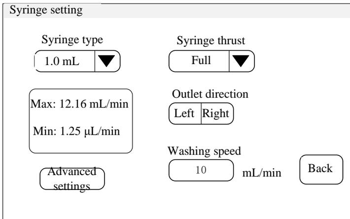
Setting syringe type, syringe thrust, outlet direction and washing speed parameter etc in this interface.
