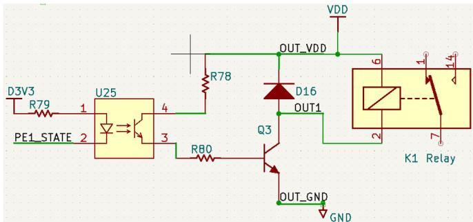
When the syringe pump starts to perform the perfusion action, the relay is closed; after the syringe pump stops the perfusion action, the relay is turned off.
