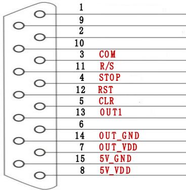
**(1) External control interface (Active signal input, 5-24VDC input)**
