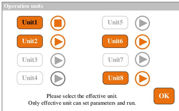
Click Operation units button in main interface, then enter to operation units interface, click Unit number button (like **Unit1**) to set unit effectiveness. After setting, click OK button back to main interface, then click start/stop button of mechanical key to control all effective unit start/stop. If a certain unit is running, and this unit is forbidden operating.
