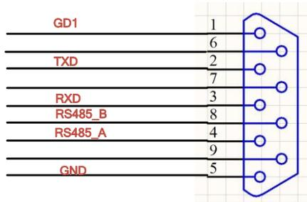
**TXD, RXD, GND:** RS232 communication interface, select RS232 in the communication setting interface, this interface is valid.
