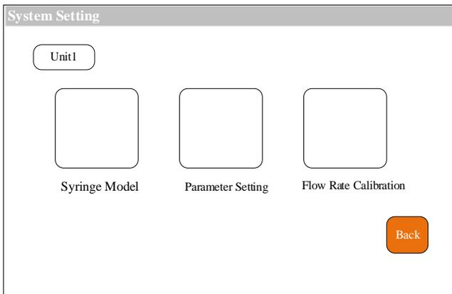
In the main interface, click the **syringe** which has been set as effective unit to enter the system settings interface. In this interface, you can choose to enter the syringe model setting interface, parameter setting interface, and flow rate calibration interface.
