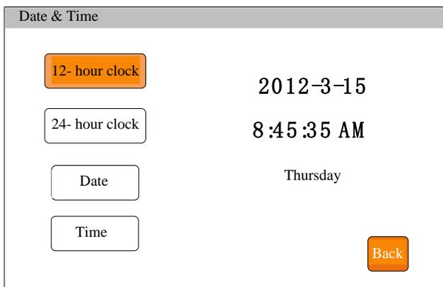
Click the **time and date** in the upper right corner of the main interface to enter the time and date setting interface. In this interface, the current date and time can be set and displayed in the upper right corner of the main interface.
